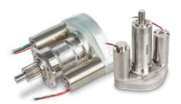
Another way of redundancy for long cylindrical motors is the coupling of two separate motors (both with own bearings) via a spur gear stage. The spur gear can be designed with 1:1 or higher ratio.
