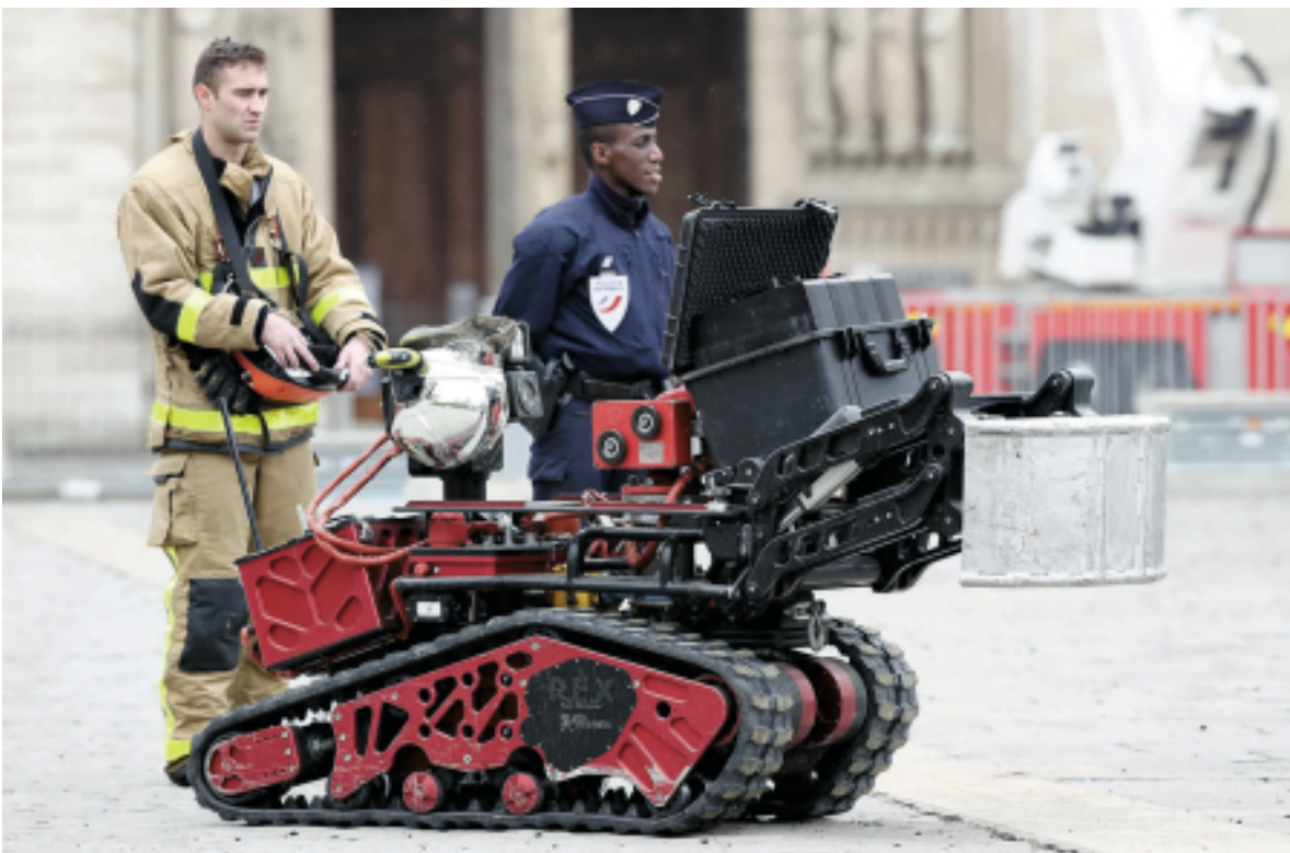
Colossus is approx. 1.6m long, 78 cm wide and 76cm tall. It weighs 500kg when empty © maxon Group
