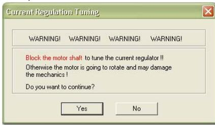
Figure 3-20 Confirmation of Shaft Blockage
