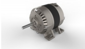
SD21 Family Torque 0.05 - 0.06 Nm Speed 1400 - 2800 RPM Power 8 - 20 Watts Voltage 12V - 240V
