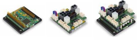
EPOS4 is a modular digital positioning controller. It is suitable for permanent magnet-activated DC motors and brushless, electronically commutated EC motors with incremental or absolute encoders with an operational range of up to 1050 W continuous power. The variety of operating modes provides high flexibility: The controllers are suitable for use in a wide range of drive systems in automation and mechatronics.
