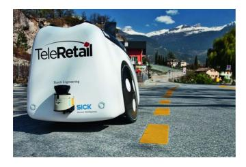
Autonomous delivery robot called the "mobile trunk" © maxon motor
