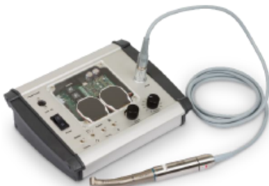
Figure 1: HPSC demo unit with dental motor
