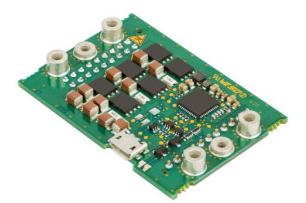
The ESCON Module 50/8 HE servo controller with and without heat sink. © maxon motor
