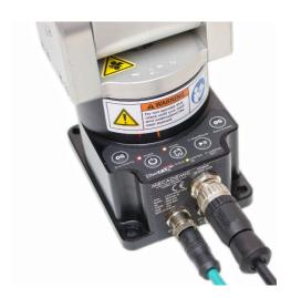
maxon motor's brushless pancake motors are available in a variety of sizes and are perfectly suited for robotic applications. The Meca500 has six degrees of freedom and weighs only five kilograms. The controller is integrated into the base.
