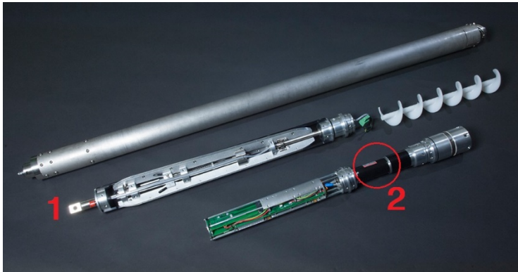
The Drill showing 1) Chipping spiral, 2) Motor controller, 3) Spinning cutter barrel, 4) Cutter, 5) Fixed chipping spiral.
