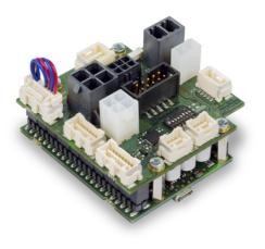
Easy to use DC motor position controller connector version © 2016 maxon motor.
