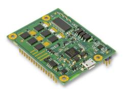
Easy to use DC motor position controller module © 2016 maxon motor.
