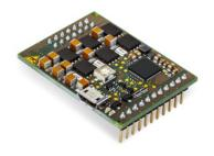
Small brushless motor control unit. The Easy to use servoamplifier.
